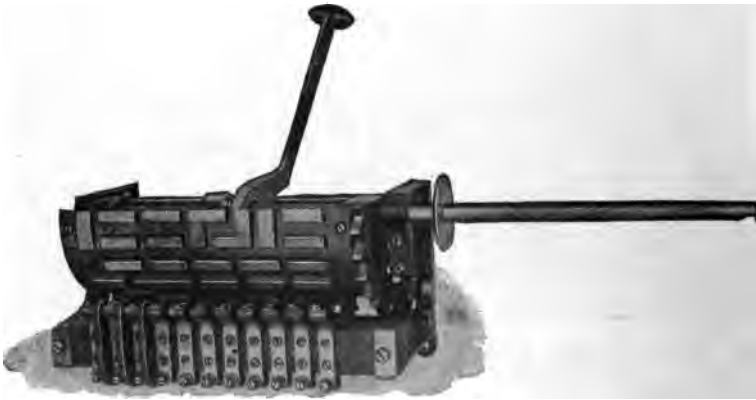
FIG. 310.—Typical Controller of the General Electric Co., showing means for making circuit connections through conducting segments on the periphery of the controller-cylinder.
